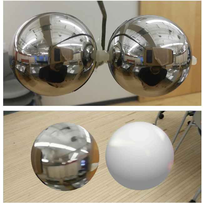
Figure 7. View from rear-facing camera (top) used to create a realistic environment map on two virtual spheres (bottom; specular and diffused reflection).
