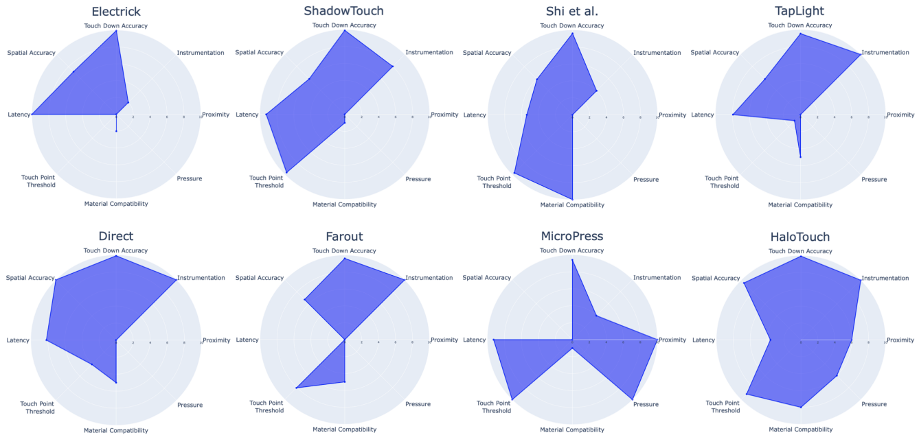
Figure 1: Radar charts comparing eight touch input systems (Electrick[69], ShadowTouch[39], Shi et al.[57], TapLight[58], Direct[64], FarOut[56], MicroPress[15], HaloTouch) across metrics like Accuracy, Latency, Material Compatibility
